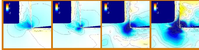
stress distribution simulated with a dynamic FEM simulator developed (in GPa)
