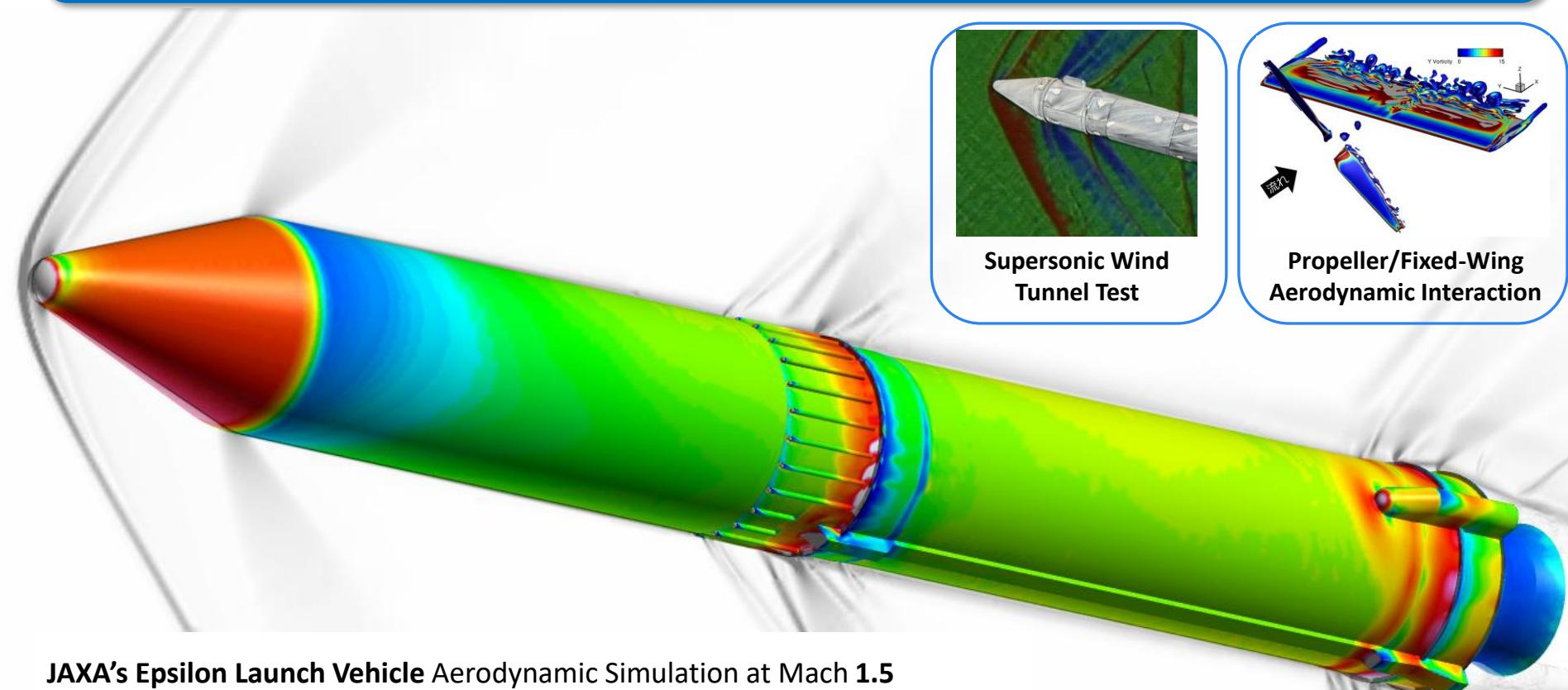
JAXA's Epsilon Launch Vehicle Aerodynamic Simulation at Mach 1.5
